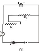
(d) In the circuit (X) the resistors R1 and R2 are connected in series while these are connected in parallel in circuit. (Y)
